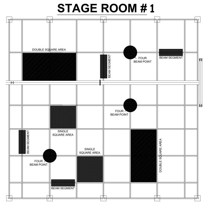
STAGE ROOM 1 & 2: STANDARD DISTRIBUTED LOADING 65#/LF ALL BEAMS STANDARD LIFTING CAPACITY OF 20 TONS SPECIAL DESIGNED ENGINEERED CAPACITY OF 30+ TONS
